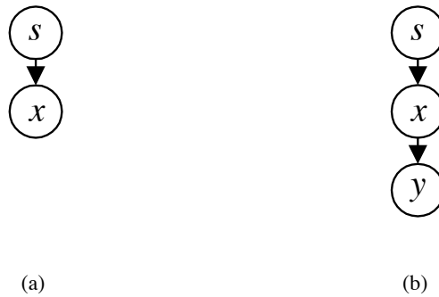
Figure 3.1: (a) Classifier for clean observations: Graph shows real valued classifier with one discrete variable s and one continuous observed variable x . (b) Classifier for corrupted observations: Graph with one discrete variable s one continuous hidden variable x and a continuous noisy observed variable y .
